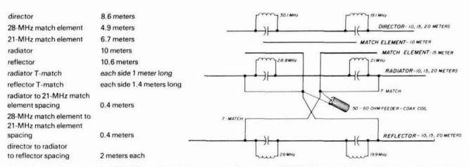
fig. 1. Physical layout of the VK2AOU multiband beam as manufactured by DJ2UT. The capacitors are formed by short lengths of coax inserted in the center of the element, while the inductances are small hairpin loops.
